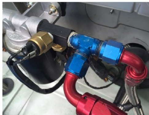
Tee-fitting shown above with the two connections (from accusump, bottom, and from the cooler, right)
