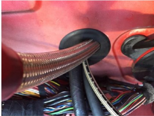
Pass the AN braided hose through the rear firewall into the trunk and connect it to the tee-fitting on the oil filter holder.
